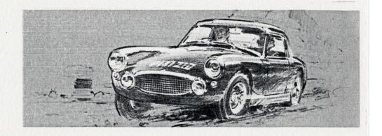
SEBRING ROAD In-line 4 cylinder OHV watercooled, three bearing counterbalanced crankshaft. Bore 2.478". Stroke 3". Cubic capacity 948 c.c. Fitted with high compression solid-skirt pistons, sports camshaft and matching distributor, three branch exhaust system and silencer, 7,000 r.p.m. valve springs. Modified inlet ports and combustion chambers 9.0 to 1 compression ratio approximately 55 b.h.p.
